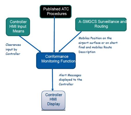
Figure 6 Conformance monitoring alerts – Ground functional architecture
