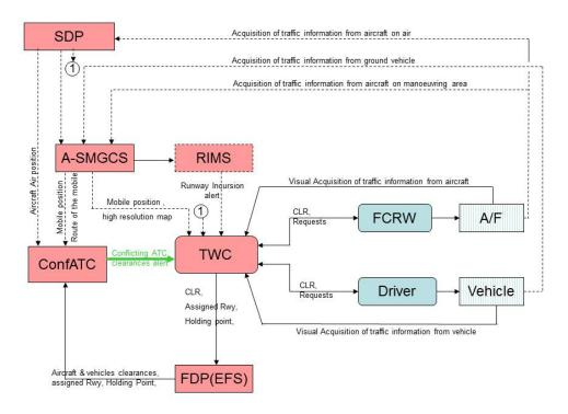
Figure 5 functional architecture of Conflicting ATC Clearance system
