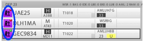
Figure 2 LED predictive information: two possible conflicting clearances indicated by a red circle in the flight strips UAE25 and DLH1MA (in the figure highlighted by blue circle) 1
