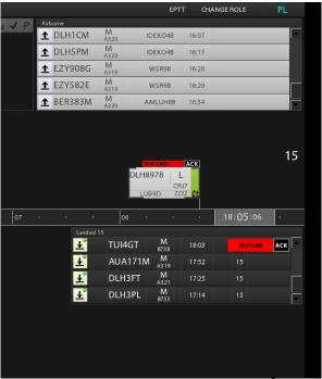
Figure 3 TOF/LND alert on FDPS
